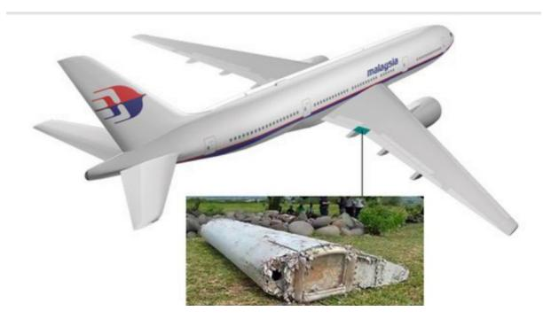
Figure 3a: Flaperon found on Reunion Island and its assembly location on a Boeing 777
